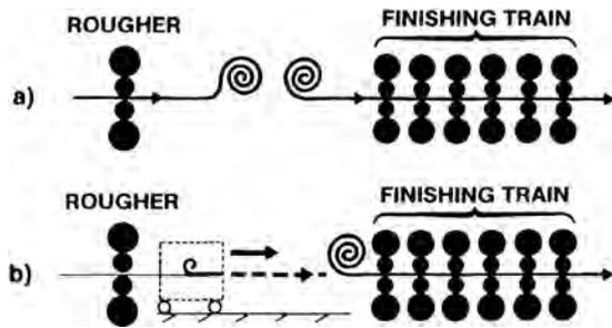
Fig. 14.15 Basic concept of Coilbox (a) and inverse arrangement (b).
